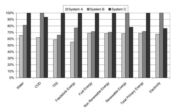
Figure 5.13 Comparison of water consumption, COD and TSS emissions and energy indicators of Systems A, B and C.
