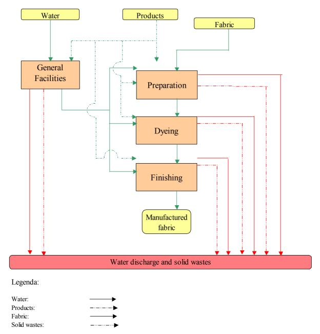
Fig. 2.1 Material flowchart of I04 company
