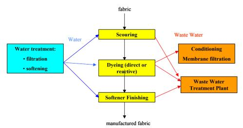
Fig.2.2 Schematic flowchart of analysed viscose fabric products
