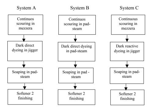
Figure 3.1 Flow-chart of the selected production lines
