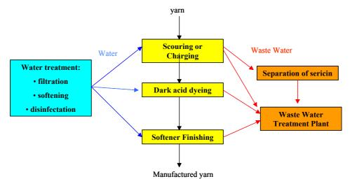
Fig.2.2 Schematic flowchart of analysed silk yarn products (Separation of sericin is missing in case of charging pre-treatment)
