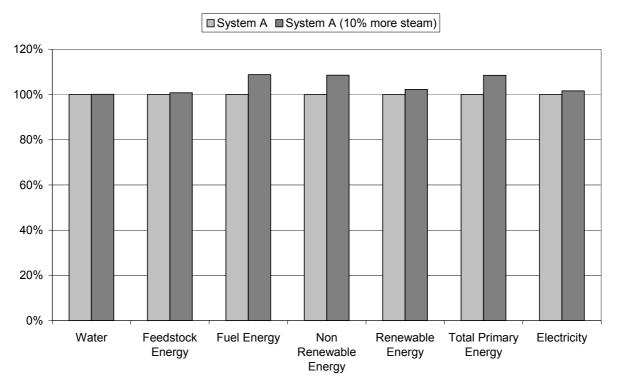
Figure 5.14 Sensitivity check of System A to the uncertainty of steam consumption
