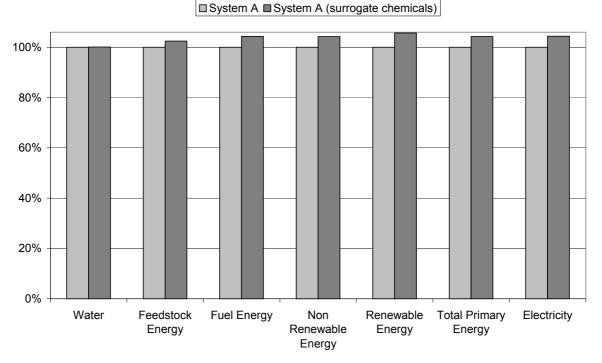
Figure 5.18 Sensitivity check of System A to lack of data about chemicals
