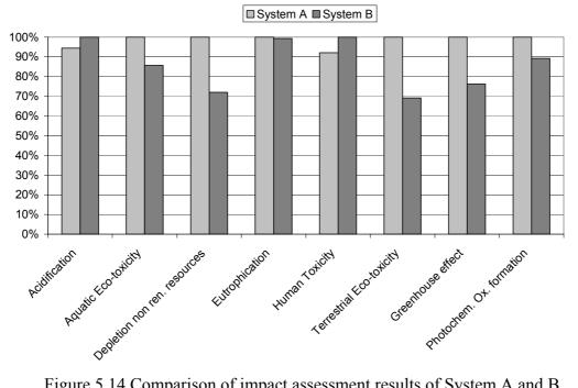
Figure 5.14 Comparison of impact assessment results of System A and B
